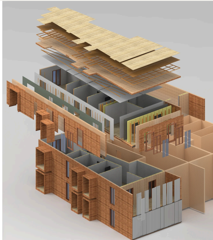
Detail: proposed housing construction layers.
